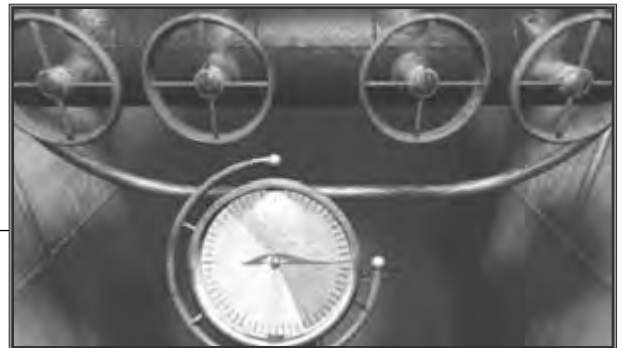
Fig. 3-26. These valves control the air pressure for inflating the airship. No hot air is flowing, however.
