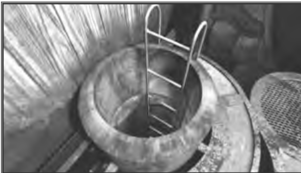
Fig. 3-11. This shaft leads down to a crank mechanism that can raise the floor gear.
