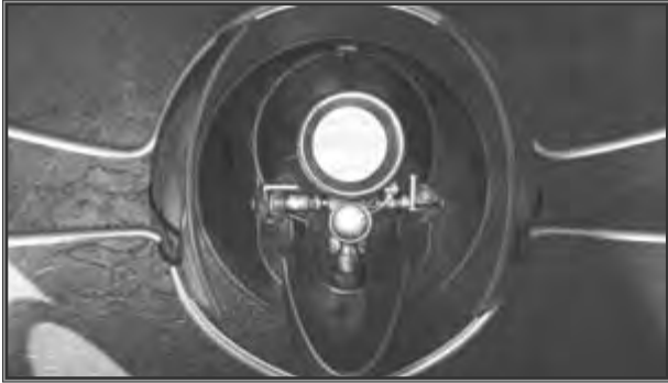
Fig. 2-27. Pan to position the tusk's symbol behind the one etched on the lens. Then use focus and zoom controls to align the two symbols (tusk and lens) precisely.
