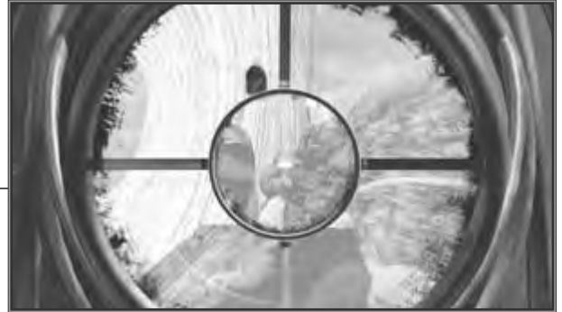
Fig. 2-38. Turn the final red pole once to direct the beam to the prism (as seen here through the view-scope).
