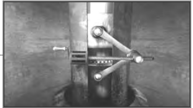
Fig. 3-12. Turn the crank handle on the left side of this mechanism to raise the floor gear.
